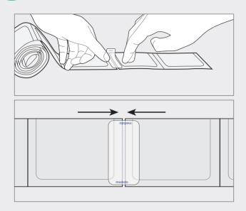
It is recommended to attach a new medication roll to the current roll when there are two pouches left.
